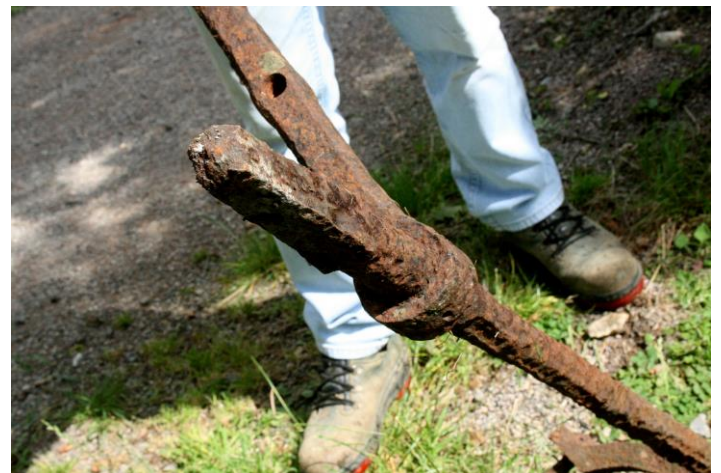
Paddle gear mechanism from Pewsham Top Lock. The windlass would have turned on this end.
