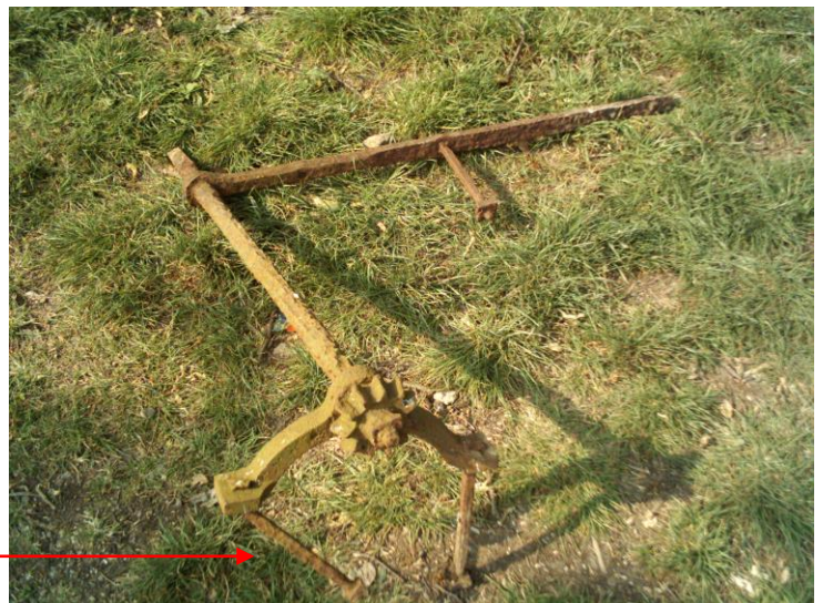
Paddle gear mechanism from Pewsham Top Lock. The windlass would have turned on this end.
